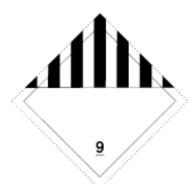
(b) In addition to conformance with §172.519, the background on the CLASS 9 placard must be white with seven black vertical stripes on the top half extending from the top of the placard to one inch above the horizontal centerline. The black vertical stripes must be spaced so that, visually, they appear equal in width to the six white spaces between them. The space below the vertical lines must be white with the class number 9 underlined and centered at the bottom.
