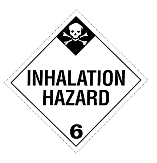
(b) In addition to complying with §172.519, the background on the POISON INHALATION HAZARD placard and the symbol must be white. The background of the upper diamond must be black and the lower point of the upper diamond must be 65 mm (25/8inches) above the horizontal center line. The text, class number, and inner border must be black.
